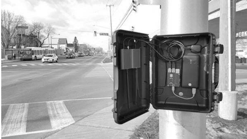
Figure 8.1: A portable Bluetooth and WiFi scanner unit secured to a roadside pole. The battery operated sensors can collect data for several days at a time. This is TrafficBox from Smatstraffic, www.smatstraffic.com .
